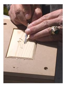
Next Charlie chisels out the waste, chiseling up to the cut line, recognize that this is a small amount of waste as the router has removed the majority of the waste around the line.
