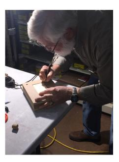
After tracing around the piece to be inlayed, Charlie uses a scalpel to cut along the line. (Notice the box is insert to a jig that is level with the box lid.)
