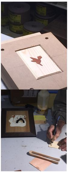
Voilà, the insert is glued into the routedout lid with the assistance of a leather pad over the inlay and some clamps.
