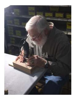
Next Charlie uses a Dremel, in a router base, with a small upward spiral bit to route just inside the line. The router depth is set with a piece of veneer under the router base. This Dremel router base can be purchased from Stewart-McDonald at www.stewmac.com.
